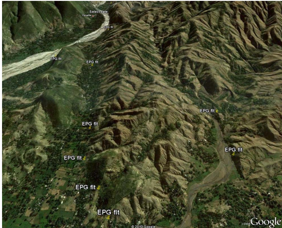
Figure 4.1. View east towards Fayette and Leogane along parallel east-northeast trending traces of Enriquillo Plantain Garden fault. Fault trace marked by push-pins labeled “EPG flt”. Fault trace at right (left offset of river along prominent north-facing scarps) apparently steps north to linear valley of Momance River at top left of picture.
