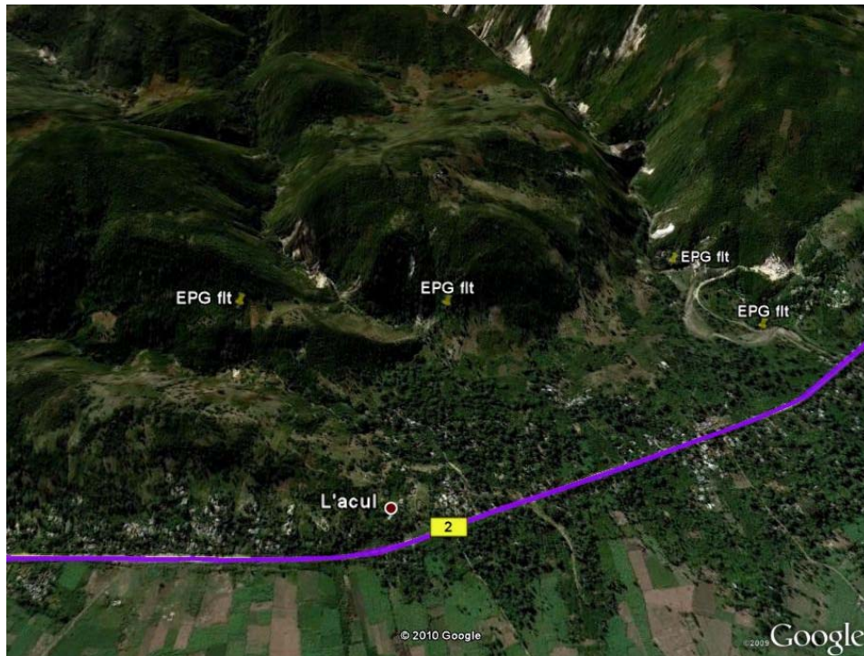
Figure 4.7. View south of shutter ridge blocking drainage (center) and offset stream channel (center right) along fault south of L’acul. Fault trace marked by push-pins labeled “EPG flt”.
